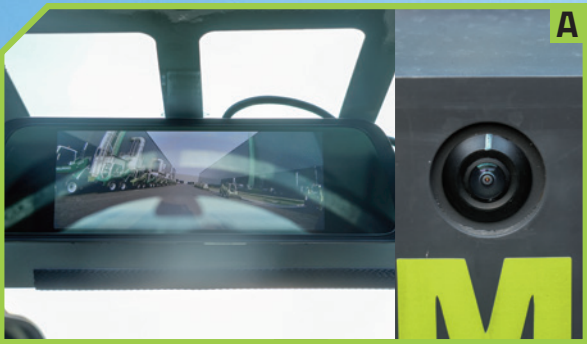
Optional reversing camera Its large display at the front of the cab and the high-definition camera at the rear ensure a complete view of the machine's rear door.
