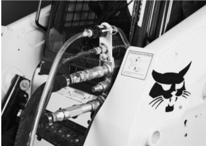
Quick-tach couplings for fast connections to attachment carrier.
