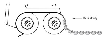
Using a rope or chain, the tracks are easily pulled over the tires by backing the loader slowly.
