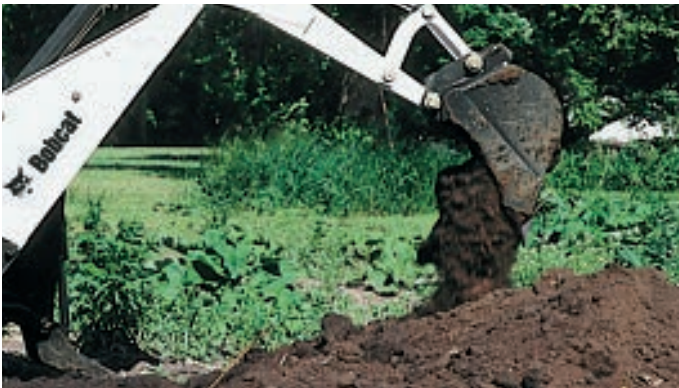
TRENCHING BUCKETS – Standard or severe-duty – severe-duty has weld-on teeth and increased steel in high-wear areas
